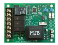
To provide maximum system efficiency the HWCB controls the compressor, fan, and reversing valve and compressor cooling solenoids. This provides total system control in a small easily adaptable package that can also be easily fitted to other brands or makes of hot water heap pump systems that may have had their control system fail.
