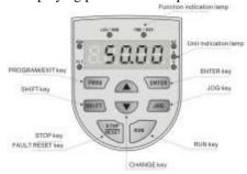
Fig. 4-1 SY7000 operation panel deployment diagram
